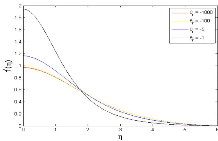
FIGURE 6. Effects of variable -viscosity parameter on velocity profiles  $f'$  when  $\lambda = -1/3, \phi = 0.02$ .
