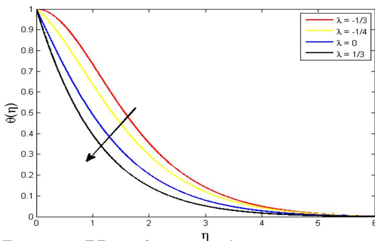
FIGURE 5. Effects of parameter  $\lambda$  on temperature profiles  $\theta(\eta)$  when  $\phi = 0.02, \theta_r = -1$ .
