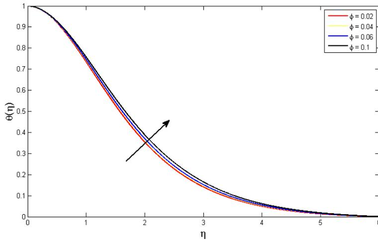
FIGURE 3. Effects of nanoparticle fraction volume on temperature profiles  $\theta(\eta)$  when  $\lambda = -1/3, \theta_r = -1$ .
