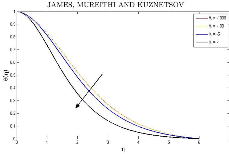
FIGURE 7. Effects of variable -viscosity parameter on temperature profiles  $\theta(\eta)$  when  $\lambda = -1/3$ ,  $\phi = 0.02$ .
