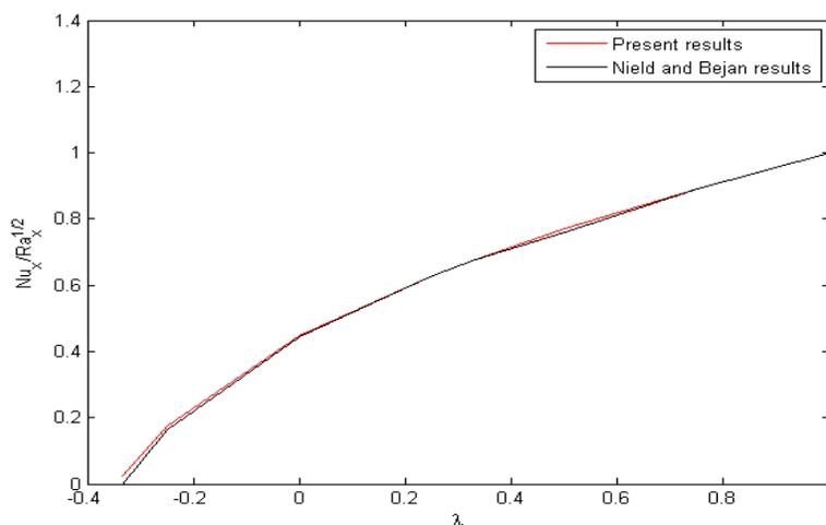
FIGURE 9. Comparison between the present results and Nield and Bejan results on the heat transfer from the heated plate when  $\phi = 0$  and  $\theta_r \rightarrow -\infty$ .
