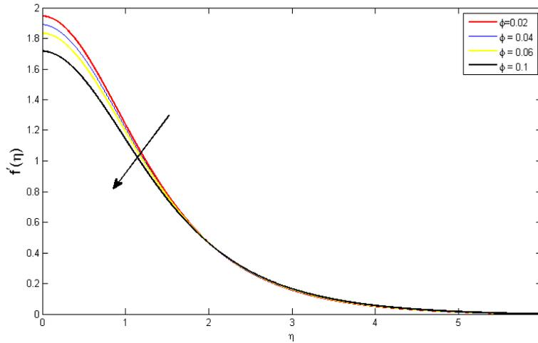
FIGURE 2. Effects of nanoparticle fraction volume on velocity profiles  $f'(\eta)$  when  $\lambda = -1/3, \theta_r = -1$ .
