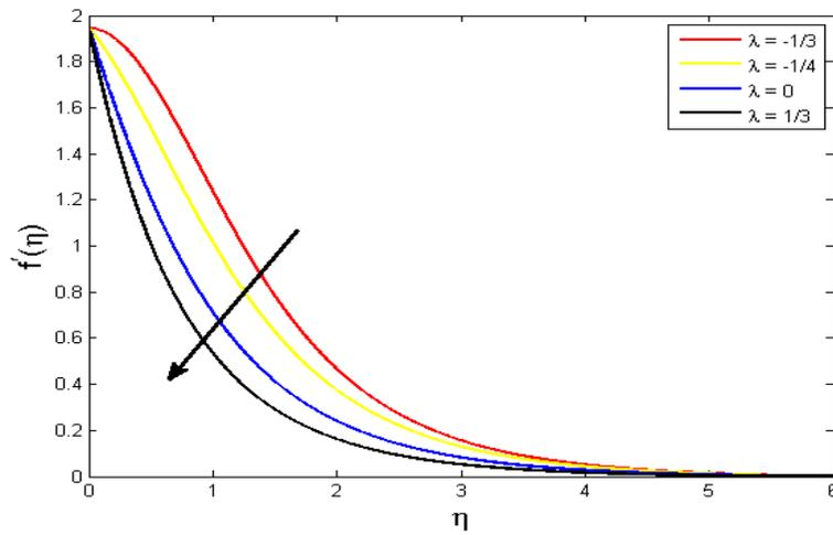
FIGURE 4. Effects of parameter  $\lambda$  on velocity profiles  $f'$  when  $\varphi = 0.02, \theta_r = -1$ .
