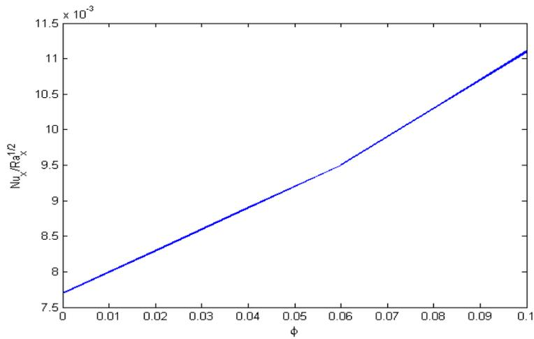
FIGURE 8. Effects of heat transfer from the heated surface for various values of nanoparticle fraction volume when  $\lambda = -1/3$  and  $\theta_r = -1$ .
